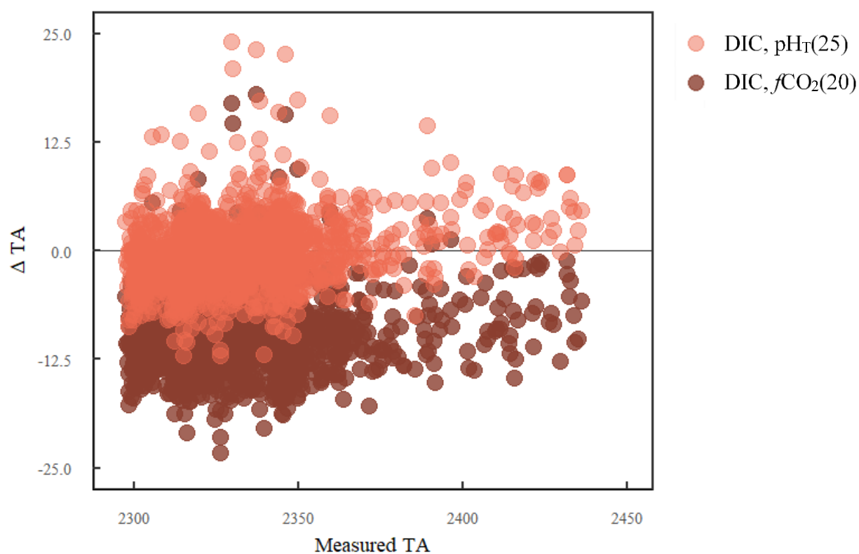
Fig. 3. Residuals of TA ( \Delta TA = \text{measured TA} - \text{calculated TA} ; \mu\text{mol kg}^{-1} ) shown in terms of measured TA. Color denotes the input pair used for TA calculations: (DIC, pH_T(25) ) or (DIC, fCO_2(20) ).
